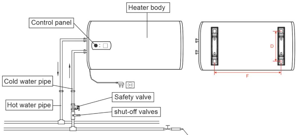
3. Install the supply socket in the wall. The supply socket should be 3 pins, single phase, 230V/16A. It is recommended to place the socket on the right above the heater. The height of the socket to the ground shall not be less than 1.8m.
